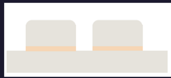
Case 2: Sufficient descum time Optimized polymer deposition
