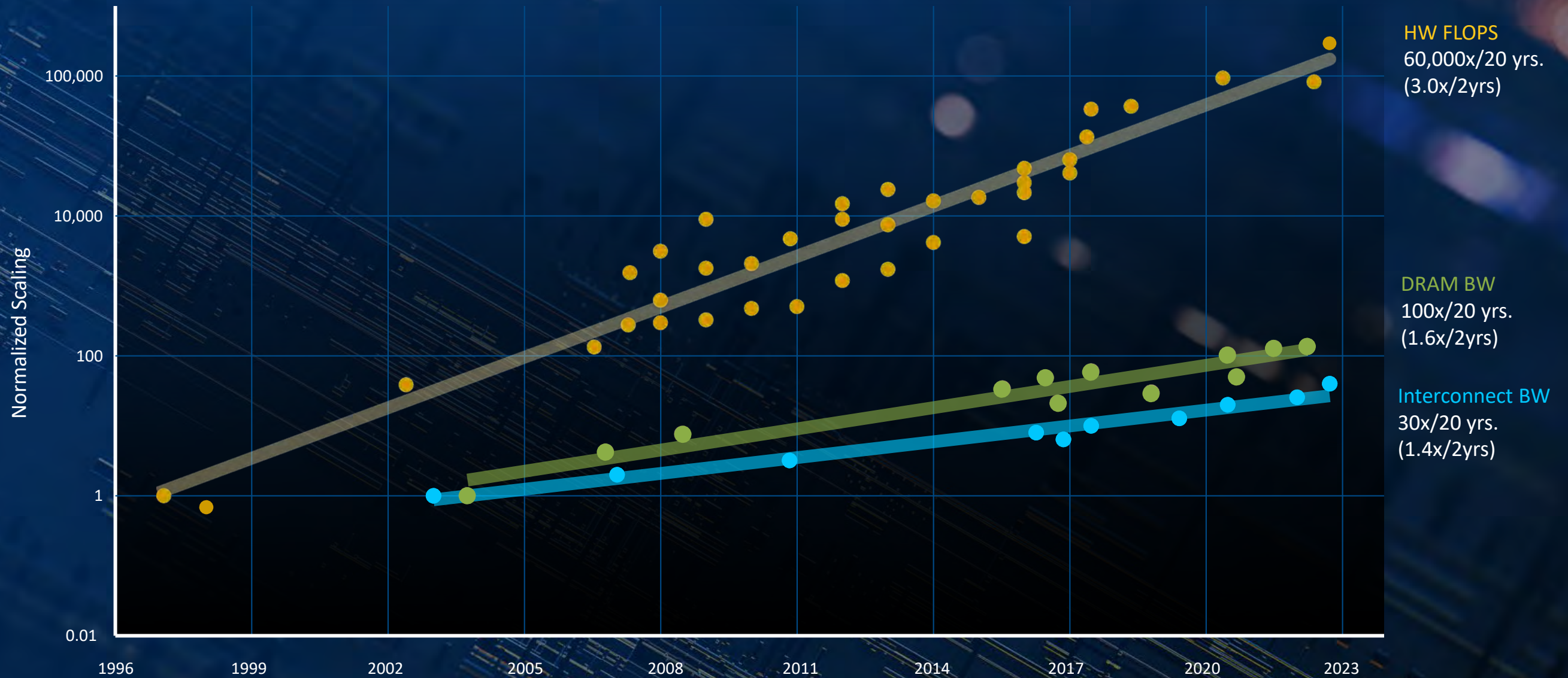
Scaling of Peak Hardware FLOPS and Memory/Interconnect Bandwidth
